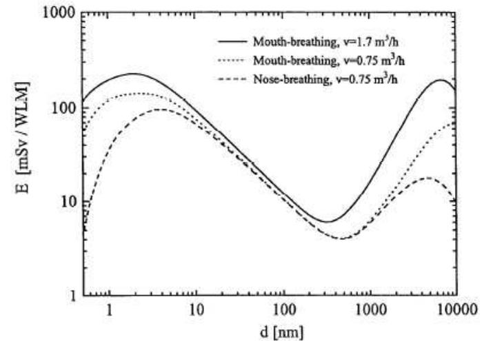
Fig. 2. DCF (in effective dose) as function of the particle diameter obtained from model calculations (Zock 1996) based on the human respiratory tract model of ICRP 66 (target tissue: secretory and basal cells;  $w_R = 20$ ;  $w_{TBB} : w_{TBL} : w_{TAL} = 0.333 : 0.333 : 0.333$ ;  $w_T = 0.12$ ).
