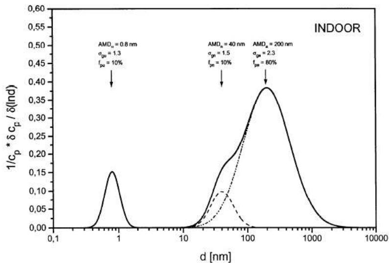
Fig. 3. Relative size distribution of the PAEC of radon daughters typical for indoor air in closed rooms of homes (without additional aerosol sources).
