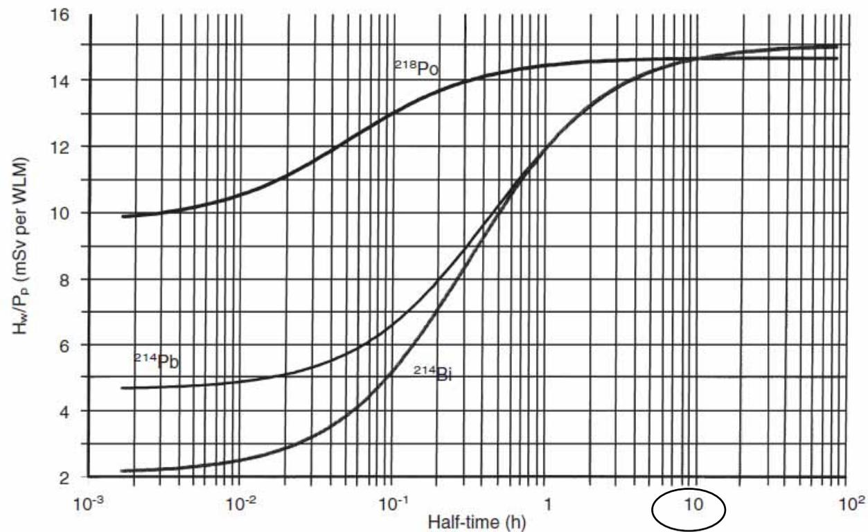
Figure 6. Sensitivity of weighted committed equivalent dose to lung per working level month ( $H_w/P_p$ ) to the absorption half-times of  $^{218}\text{Po}$ ,  $^{214}\text{Pb}$  or  $^{214}\text{Bi}$ .
